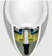
The centrepiece of the uridan® urinals is the patented uridan® odour trap: This odour trap works with the aid of uriLOCK®, a special blocking fluid. uriLOCK® consists of plant-based substances and is biodegradable. Due to the fact that it is lighter than urine, the heavier urine automatically flows directly down the drain. The lighter uriLOCK® stays on the surface and works like a liquid lid that blocks out all drain and sewage odours.
